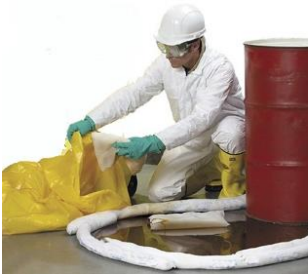
Figure 2: Example of spill kit contents being used to contain a leak
